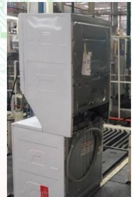
Washing center seen on the back face, the exhaust is located in the middle part.
