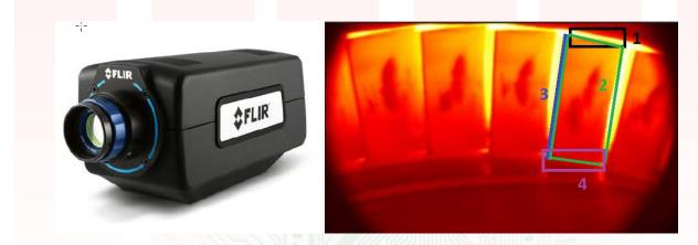
It is necessary to be able to access to a direct view of the blade with the cameras through a window or peephole. In this case, by means of a camera in the near infrared (SWIR) it is possible the inspection in real time, realizing a precise synchronization, with a team like the Key-Phasor of Bentley Nevado.
