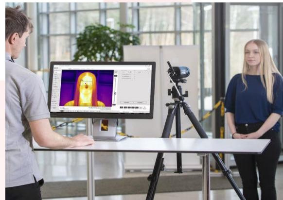
A500-EST camera connected directly to monitor display (courtesy of FLIR Systems)
