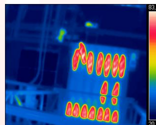
Tray with a loaf displaced from its ROI and zone without loaves
