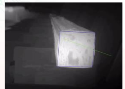
Tail of a billet with the result of inspection and dimensional control.
